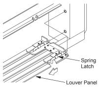
Figure 40 - Removing Louver Panel
